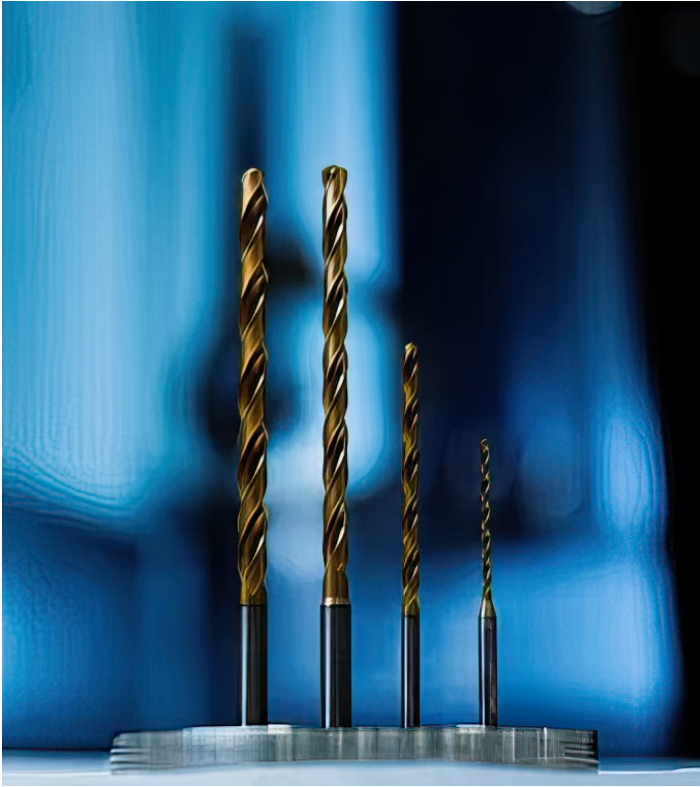
▲ Kennametal's KenDrill HPR solid carbide drills use a patented corner radius to extend tool life while achieving high hole quality. The corner radius also helps avoid chipping the workpiece during part exits.
