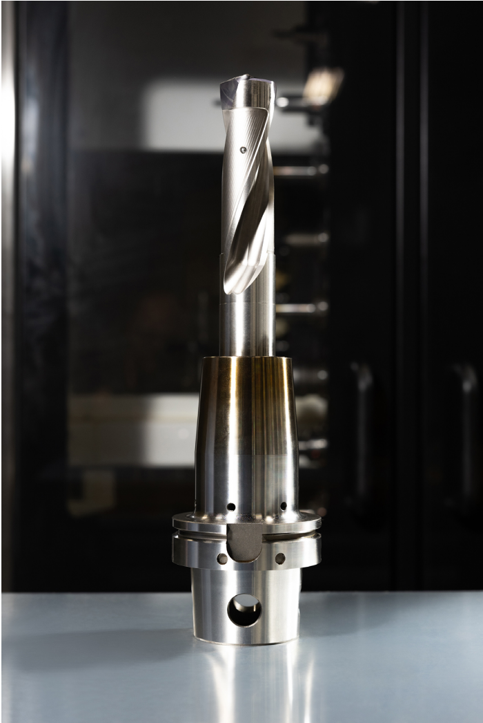
▲ KSEM modular drills feature material-specific point geometries for compatibility across many materials. They also sport an internal coolant supply, which directly hits the cutting zone to improve chip evacuation and tool life.
