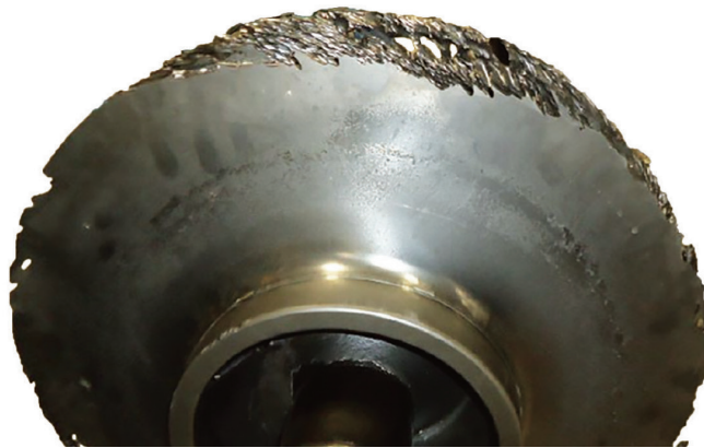
13 个月 after 泵叶轮无 Conforma Clad 防护
