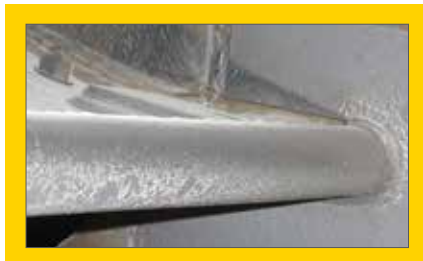
Fan blade protected with Conforma Clad liner.
