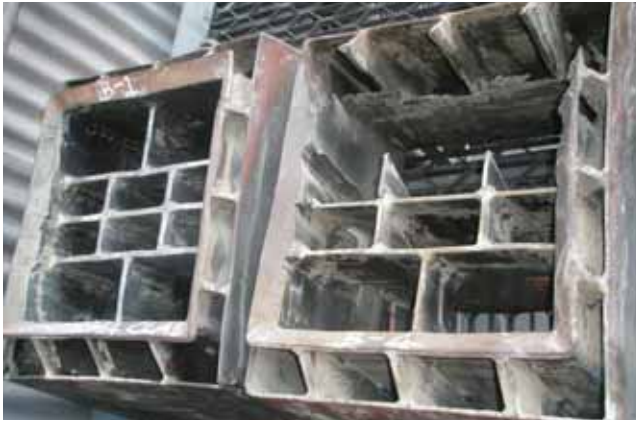
Side by side comparison (boiler side view) of the weld overlay protected coal nozzle tip (right) and the Kennametal tip (left).
