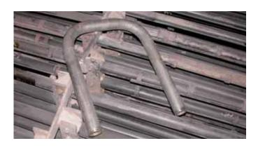
Kennametal infiltration brazed cladding measured by eddy-current revealed thickness loss, in a localized area, in line with a catalyst injection nozzle at 0.002; remaining clad area had no measurable coating thickness loss.
